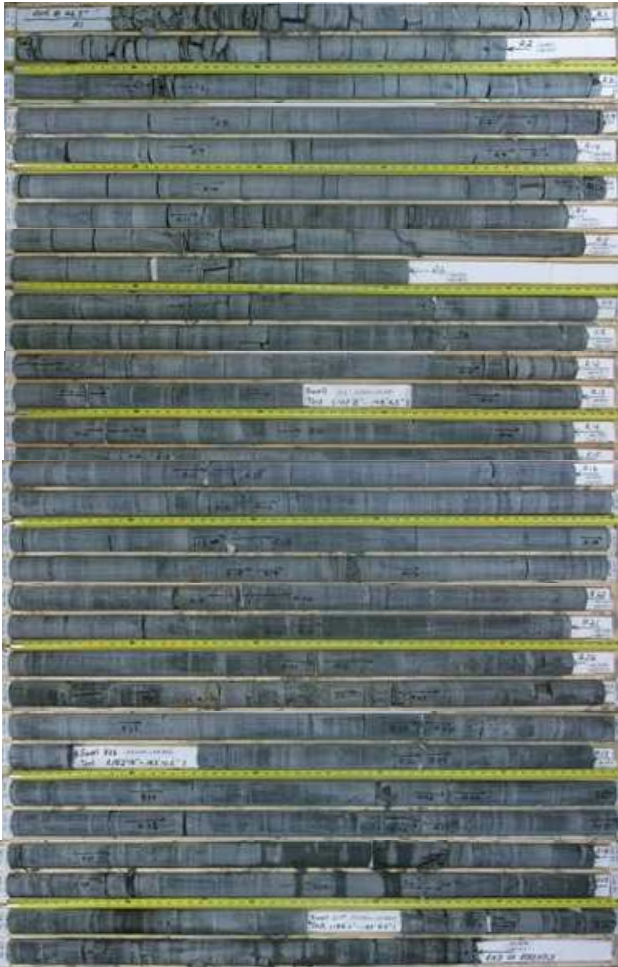
Figure 1. Photographs of rock cores taken at depths of 14.2 m to 59.5 m below the existing ground surface at Location 4
